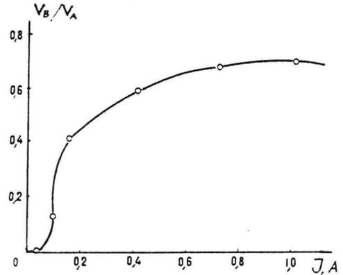
Fig. 6. Relation between attenuation of incoming flow velocity in the roughness edge centre (point A) and current in channel I (experimental data).  $V_b/V_a=f(I)$ , where  $V_a$  - flow velocity in point A,  $V_b$  - flow velocity in point B, located on the 'roughness stern', i.e., after flow has passed the roughness. The instrumentation equipment - see Fig. 5.
