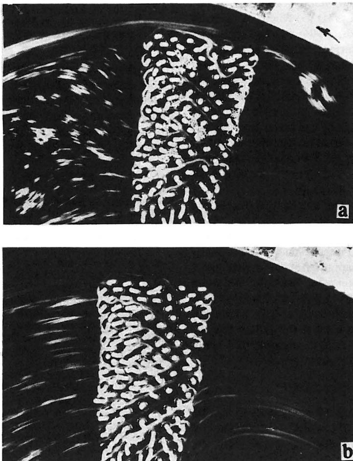
Fig. 5. Photos of electrolyte flow structure formed as a result of its interaction with limited-size model of homogeneous vegetation. Diaphragm 5.6; exposure time 4 s; film MIKRAT-300. a)  $I=100$  mA b)  $I=400$  mA. The model of roughness is located in channel II (see Fig.2).
