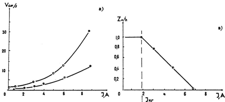
Fig. 4. Relation between flow velocities (a) and level of turbulent flow permeability in the model of vegetation  $z_0/h$  (b) and current  $I$ . 1.  $V=f(I)$  at  $z=r_{av}+h$ . 2.  $V=f(I)$  at  $z=h$ .
