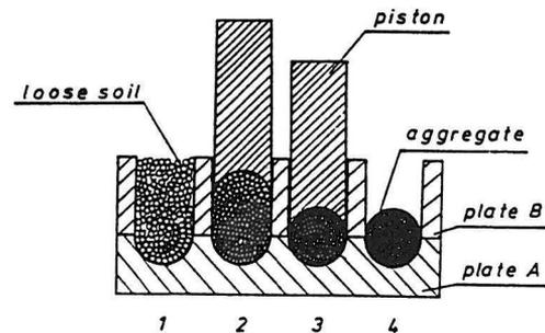
Fig. 1. Diagram of the device for aggregate production showing stages of the process (1-4). The presented device concerns 15 mm aggregates (size 1:1). The devices contained 1, 10, 20, and 50 positions (holes) for the 23, 15, 10, and 6 mm aggregates, respectively. To prevent sticking of the aggregates to the piston they were covered with a thin polyethylene foil.
