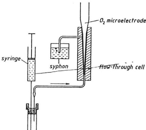
Fig. 3. Diagram of the system used for pushing air samples from the incubation jar with water filled syringe to oxygen microelectrode installed in a flow-through cell in order to determine soil respiration rate.
