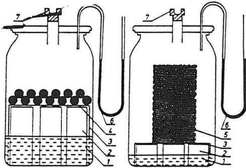
Fig. 2. Diagram of the incubation jars for the aggregates (left) and for the control (right). 1 - water, 2 - table supporting moisture tension plate, 3 - glass fiber tissue covering the table and immersed in water, 4 - soil aggregates, 5 - cylindrical nylon basket with the loose soil material <2 mm, 6 - mercury manometer, 7 - septum for gas sampling.
