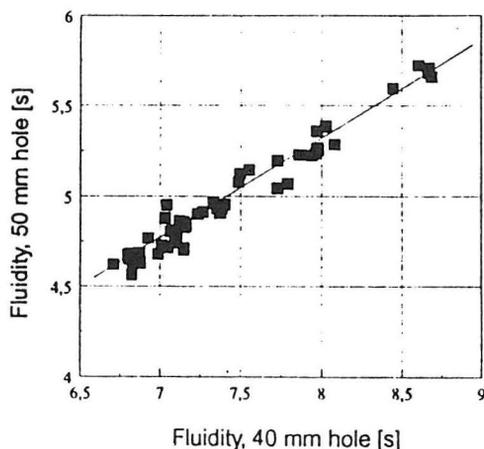
Fig. 7. The relationship between fluidity as measured with the 50 mm hole and with the 40 mm hole.
