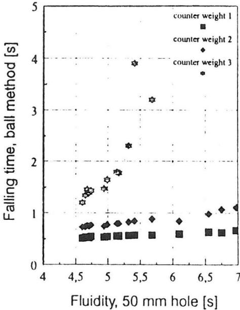
Fig. 8. The relationship between fluidity as measured with the fluidimeter (50 mm hole) and with the ball method. The three counter-weights give the ball a net bulk density of 3, 5 and 7 kg/dm<sup>3</sup>, respectively.
