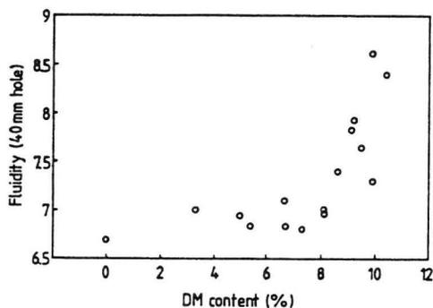
Fig. 6. The relationship between fluidity (measured with the 40 mm hole) and the DM content.
