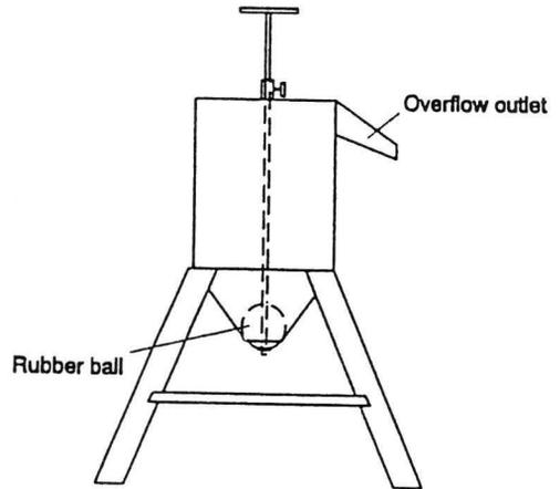
Fig. 1. The fluidimeter developed at JTI. The volume is 15.5 l and the outlet hole  $\varnothing 50$  mm. The hole can be easily changed to  $\varnothing 40$  mm using an additional cone.
