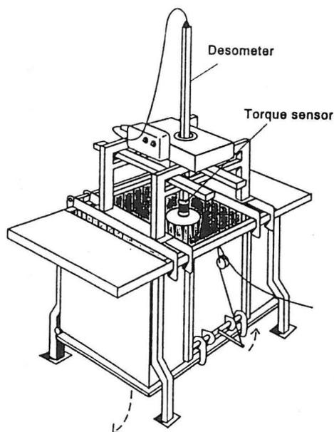
Fig. 5. The characterization box for non-pumpable manure. The box holds 1.3 m<sup>3</sup> of manure and weighs 480 kg with and 300 kg without the lifting stand. The desometer plate is 250 mm in diameter and has six 100 mm long spikes underneath.
