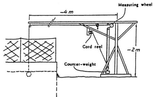
Fig. 2. The ball method. The hollow steel ball ( $\varnothing 82$  mm) is filled up with lead pellets to a bulk density of slightly more than  $7 \text{ kg/dm}^3$ . Using three different counter-weights, the ball can be counterbalanced to reach net weights corresponding to the bulk densities  $3, 5$  and  $7 \text{ kg/dm}^3$ .
