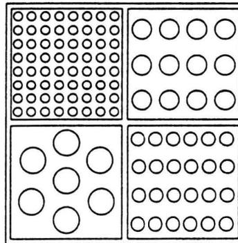
$\varnothing$  45,5 mm. Hole area,  $\varnothing$  24,5 mm. Hole area,
