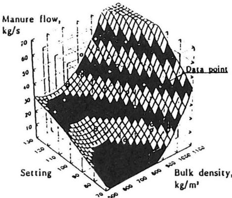
Fig. 14. The relationship between bulk density, setting and 'constant level manure flow' for a Kidd Tankspread 1500.
