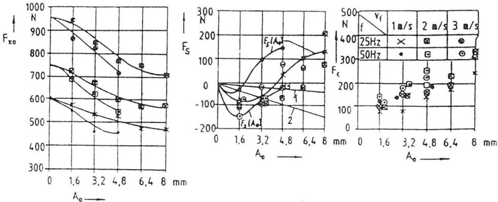
Fig. 3. Pull force  $F_{x0}$ , amplitude of damping force  $F_s$  and amplitude of spring force  $F_c$ , with the mode of operation being  $b_e$ , as a function of the travelling speed  $v_f$ , frequency  $f$ , amplitude  $A_o$  (curve 1:  $F_{sF}(A_o)$  for  $f_e=25$  cpm, curve 2:  $F_{sF}(A_o)$  for  $f_e=50$  cpm,  $\sigma=10^\circ$ ,  $l_w=75$  mm,  $b_w=250$  mm,  $l_a=100$  mm,  $l_R=575$  mm, other parameters according to Table 1).
