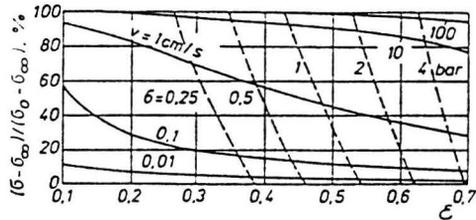
Fig. 8. Effect of loading velocity on the instantaneous pressure as a function of strain.
