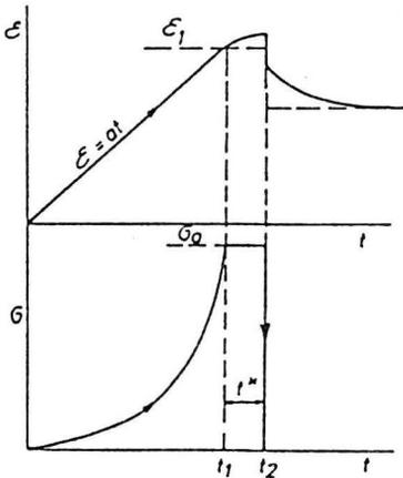
Fig. 2. Creep and rebound of the compressed material.
