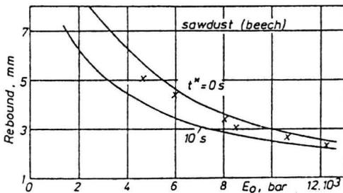
Fig. 9. The rebound of the pressed sawdust.
