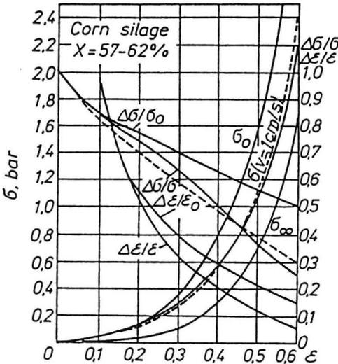
Fig. 4. Stress lines, relative relaxation and creep as a function of strain.
