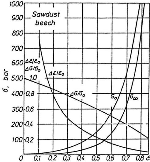
Fig. 7. Compression of sawdust as a function of strain (beech).
