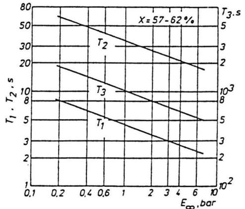
Fig. 5. Multiple relaxation times as a function of asymptotic modulus of elasticity.
