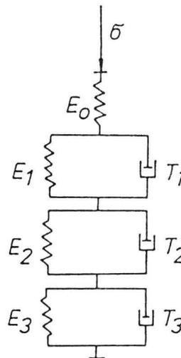
Fig. 1. The extended three-element model.
