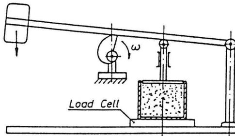
Fig. 3. Loading device for fast loading velocities.
