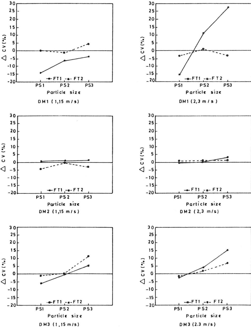
Fig.4. Based on the original commercial fertilizer, the variation of CV% in terms of the particle size.
