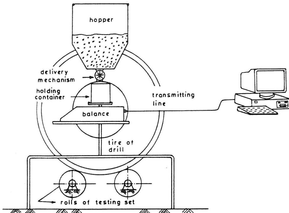
Fig. 2. Measurement setup.
