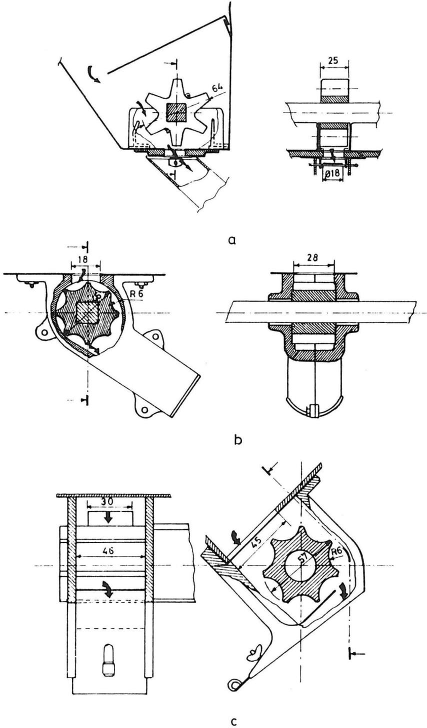
Fig.1. Fertilizer delivery mechanisms: a) with agitator wheel and adjustable gate opening; b) fluted-wheel of which effective length is unchangeable; c) fluted-wheel of which effective length is changeable.
