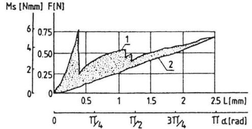
Fig. 2. Torsion curve of the pod: 1 - curve obtained in first torsion (intact pod), 2 - curve obtained in second torsion of the same pod,  $M_s$  - torque,  $F$  - registered force,  $\alpha$  - torsion angle,  $L$  - calculated linear deformation.
