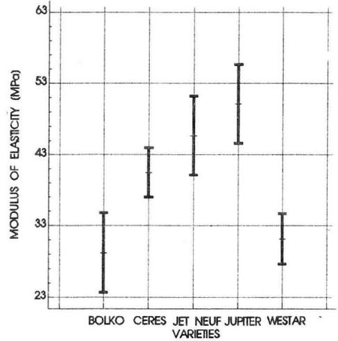
Fig. 9. Means and confidence intervals of seed modulus of elasticity.
