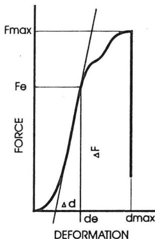
Fig. 3. Typical compression curve of a single seed with a scheme of modulus of elasticity calculation.
