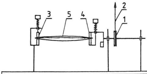
Fig. 1. Scheme of pod fixed in torsion handle: 1 - wheel, 2 - cord, 3 - immovable jaw, 4 - rotation jaw, 5 - pod.
