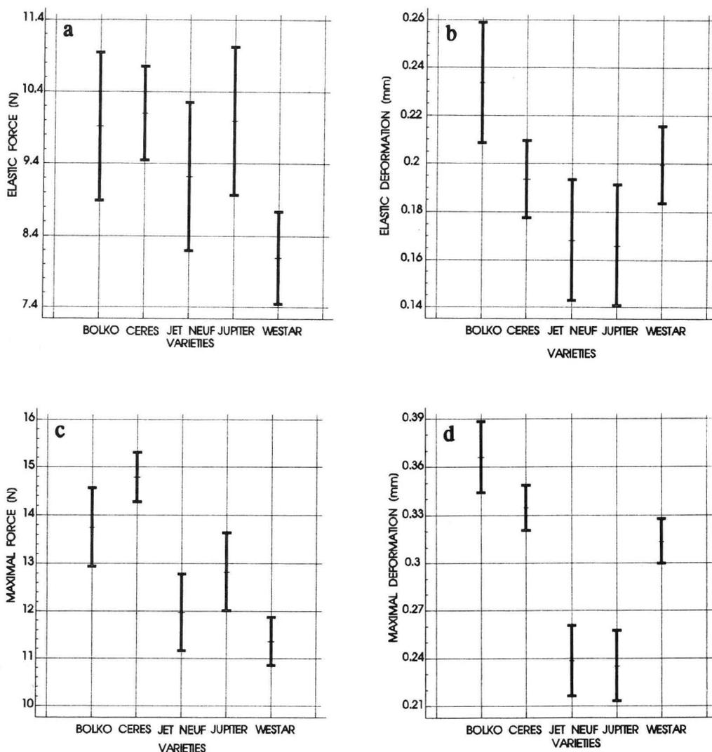
Fig. 7. Means and confidence intervals of compression elastic force (a), elastic deformation (b), maximal force (c) and maximal deformation (d).
