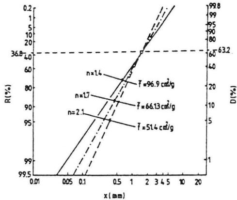
Fig. 2. Typical Rosin-Rammler distributions on RRSB-net, while  $x_0=\text{const.}$  and  $n$  parameter varies.
