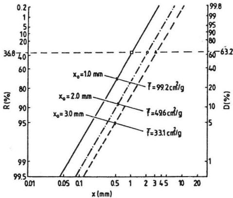
Fig. 1. Typical Rosin-Rammler distributions on RRSB-net, while  $n=\text{const.}$  and  $x_0$  parameter varies.
