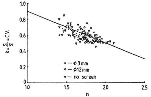
Fig. 4. The relationship of the coefficient of variation  $C.V.$  and Rosin-Rammler's uniformity coefficient  $n$  with barley grinds.
