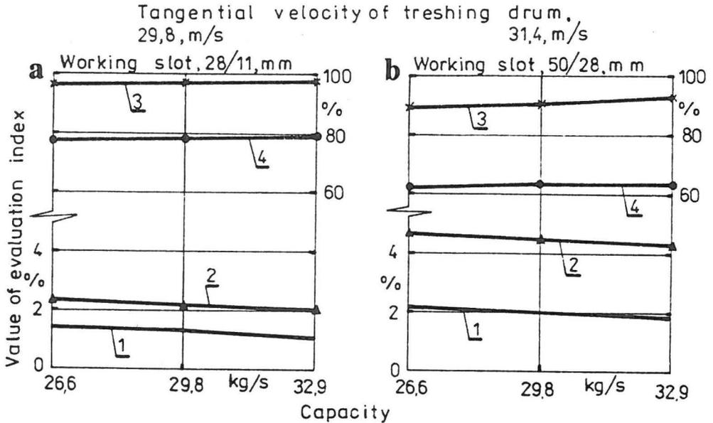
Fig. 4. Influence of capacity of the threshing set on value of evaluation index of wheat grain Emika variety (mean from 5 years of research): a - Bizon Z058, b - Bizon Z110, 1 - macro-damage, 2 - micro-damage, 3 - germination capacity, 4 - vigour of growth.
