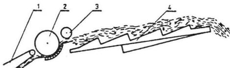
**Fig. 1.** The scheme of a traditional threshing and separating set of a combine harvester Bizon Z058: 1 - inclined conveyor, 2 - flail threshing set, 3 - straw thrower, 4 - key shaker.
