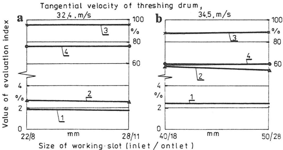
Fig. 5. Influence of size of the working slot on the value of evaluation index of wheat grain Emika variety with the capacity  $Q=2.5$  kg/s (mean from 5 years of research): a - Bizon Z058, b - Bizon Z110; 1 - macro-damage, 2 - micro-damage, 3 - germination capacity, 4 - vigour of growth.
