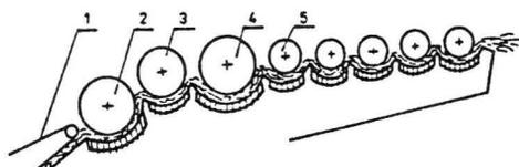
Fig. 2. The scheme of threshing and separating set without shakers in a combine harvester Bizon Z110: 1 - inclined conveyer, 2 - flail threshing set, 3 - straw thrower, 4 - threshing up and separating drum, 5 - five-drum rotary separator.
