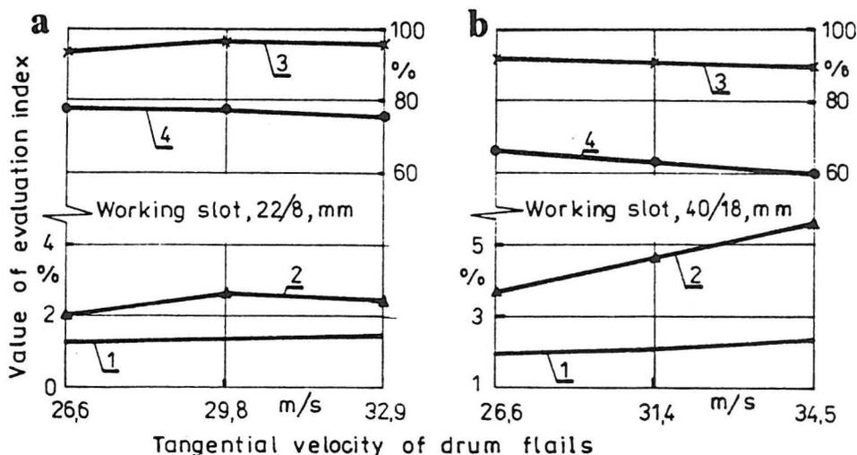
Fig. 3. Influence of tangential velocity of threshing drum flails on value of evaluation index of wheat grain Emika variety with the capacity  $Q=4.5$  kg/s (mean from 5 years of research): a - combine-harvester Bizon Z058, b - combine-harvester Bizon Z110 ; 1 - macro-damage, 2 - micro-damage, 3 - germination capacity, 4 - vigour of growth.
