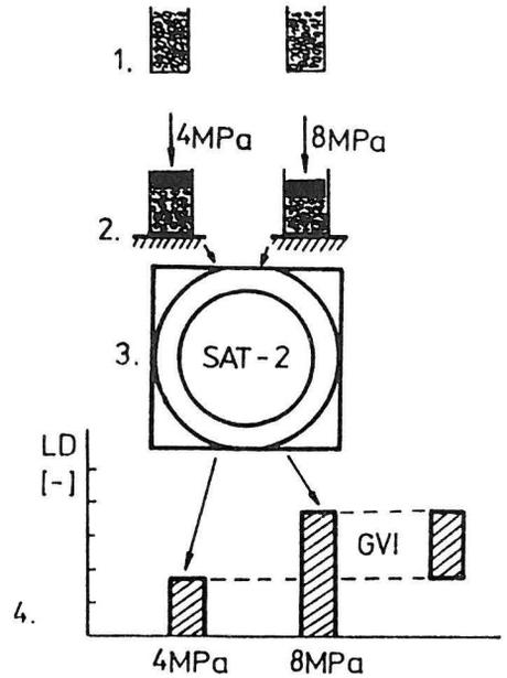
Fig. 2. Scheme of the determination of the GVI value: 1-two homogeneous grain samples, successively filling the measurement cylinder (SGD-2), 2-simulation of mechanical damage to grain (SDG-2), 3-colorimetric testing of the damage (SAT-2), 4-calculation of the GVI value.
