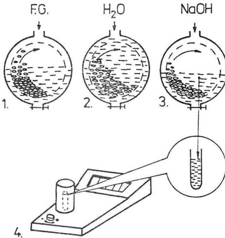
Fig. 1. Scheme of the colorimetric method: 1-soaking of the grain sample in the dye, 2-washing up of the dye excess, 3-re-soaking (test solution), 4-the measuring of the optical density in the tested solution.
