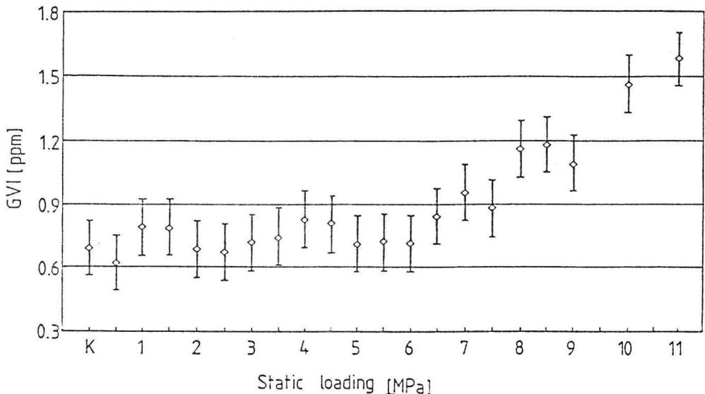
Fig. 5. Relationship between the static loading of the wheat grain sample and the value of its hardness measured by GVI.
