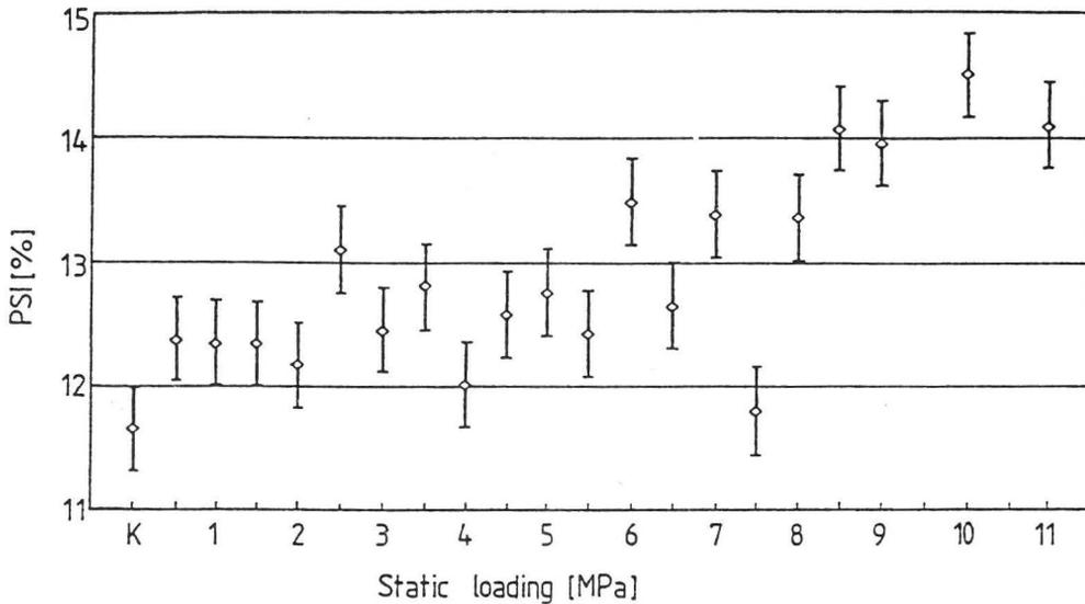
Fig. 4. Relationship between the static loading of the wheat grain sample and the value of its hardness measured by PSI.
