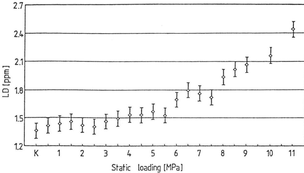
Fig. 3. Relationship between the static loading of the wheat grain samples and the value of its damage.
