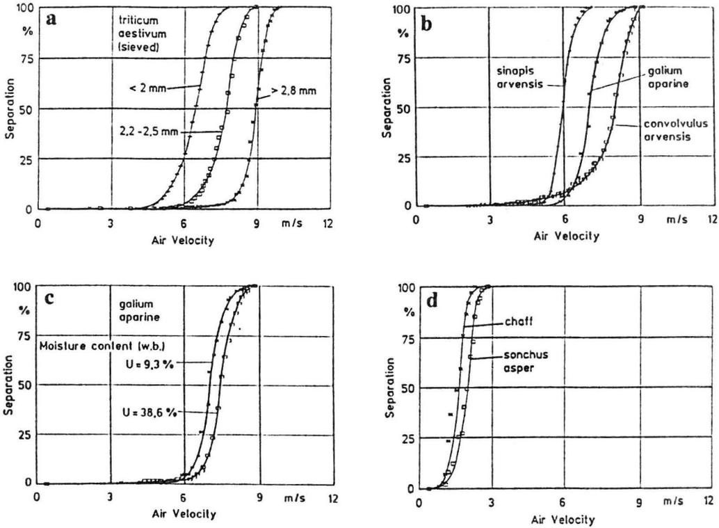
Fig. 2. Characteristic lines of suspension: a - of three different fractions of *Triticum aestivum*, b - of *Sinapis arvensis*, *Galium aparine* and *Convolvulus arvensis*, c - of *Galium aparine* at different moisture content (wet basis), d - of chaff and *Sonchus asper*.
