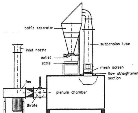
**Fig. 1.** Automatic Test Stand for determining terminal velocity of bulk material.
