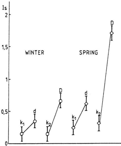
**Fig. 4.** Mean values of the indexes of damage  $I_s$  for grain samples of winter and spring wheat varieties before ( $k_1, k_2$ ) and after loading (d,D). 95 % Tukey HSD=0.21.
