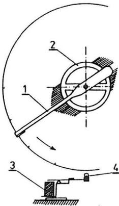
Fig. 1. Schematic diagram of the dynamic loading apparatus: 1 - rotary arm, 2 - motor with ejection control mechanism, 3 - electromagnetic ejector, 4 - kernel.
