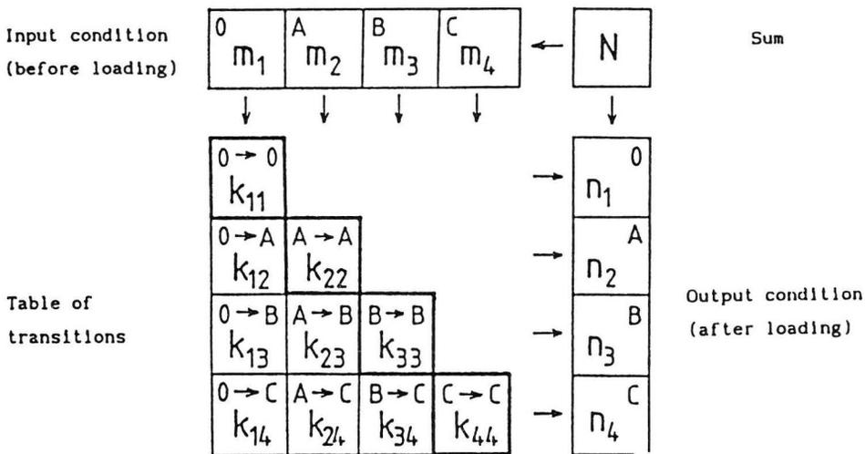
Fig. 3. Grain sample damage balance.  $N$  - size of grain sample tested;  $i, j$  - numbers of columns and rows;  $m_i, n_i$  - numbers of grains in damage classes, input and output;  $k_{ij}$  - numbers of grains in the 'windows' of the table of transitions.
