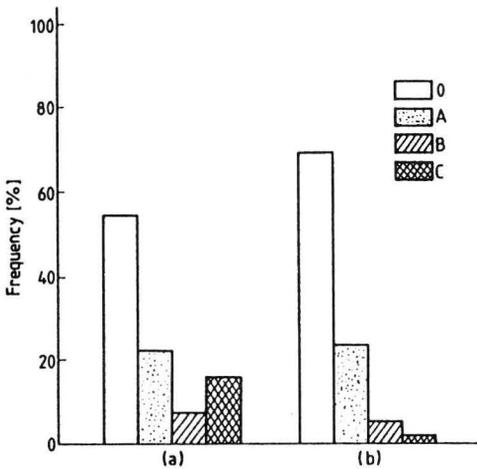
Fig. 6. Histograms of typical distributions of the damage index with respect to the grain damage classes {0, A, B, C} for Jara (a) and Liwilla (b) varieties (after dynamic loading).
