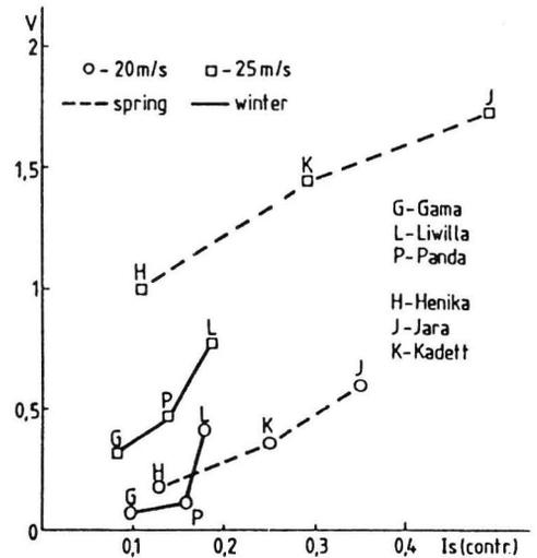
**Fig. 5.** The relation of the vulnerability index (V) to the initial status of grain damage  $I_s(\text{contr.})$  for two levels of loading within the groups of winter and spring wheat varieties.
