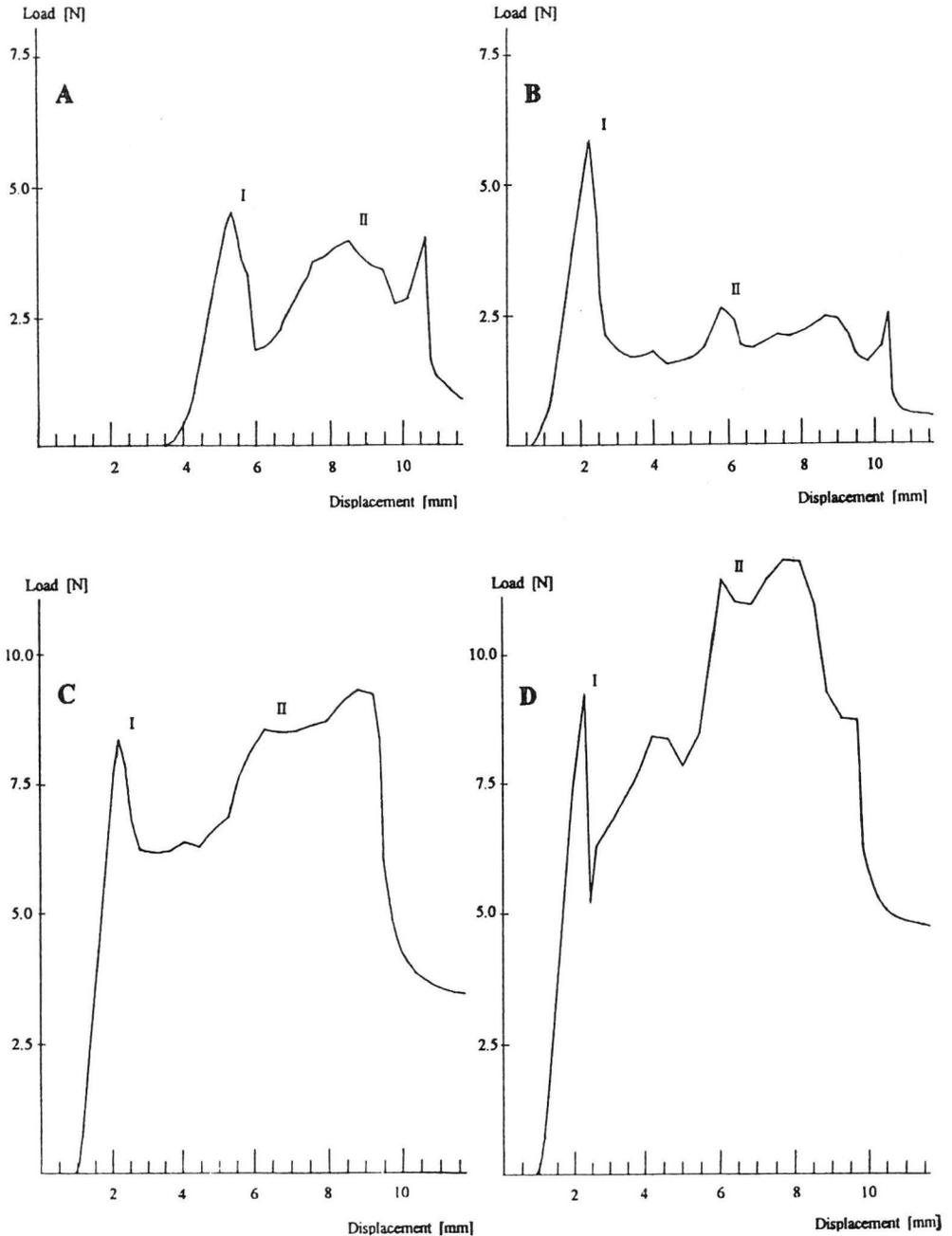
**Fig. 1.** Typical puncture test patterns of green pea seeds for Polar (A and C) and Verona (B and D) varieties: I - seed coat puncture; II - first cotyledon puncture; A and B - 19th day after flowering; C - 33rd day after flowering; D - 38th day after flowering.
