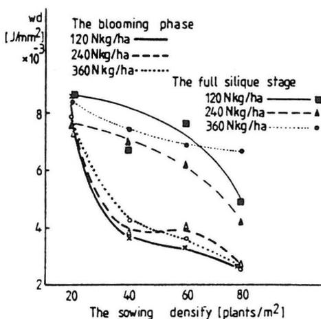
Fig. 2. The variability of shearing energy per unit of cross section area ( $wd$ ) of Jupiter winter rape stalk for different sowing density and nitrogen fertilization at two phenological phases.
