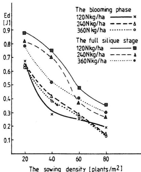
Fig. 1. The variability of shearing energy ( $Ed$ ) of Jupiter winter rape stalk for different sowing density and nitrogen fertilization at two phenological phases.
