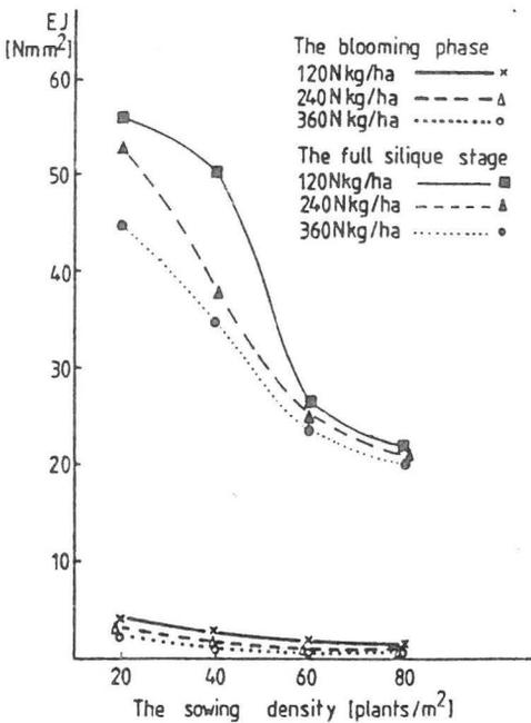
Fig. 3. The variability of rigidity ( $EJ$ ) of Jupiter winter rape stalk for different sowing density and nitrogen fertilization at two phenological phases.
