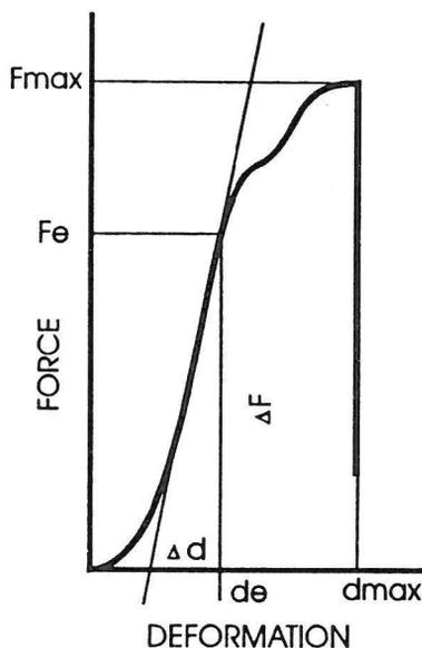
Fig. 2. Compression curve in force-deformation coordinate system and a scheme of calculation of apparent modulus of elasticity.
