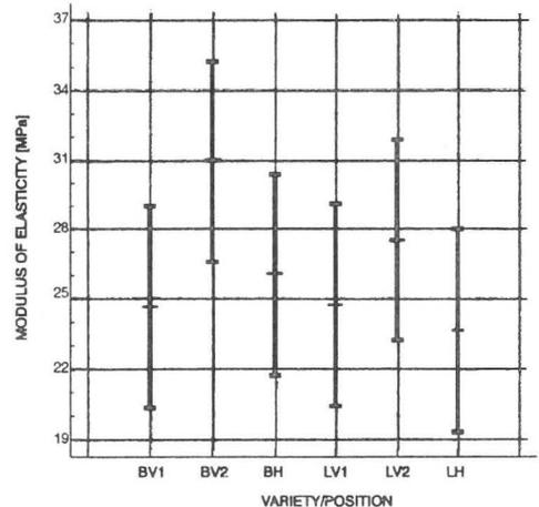
Fig. 5. Mean values with confidence intervals of apparent modulus of elasticity of seeds.
