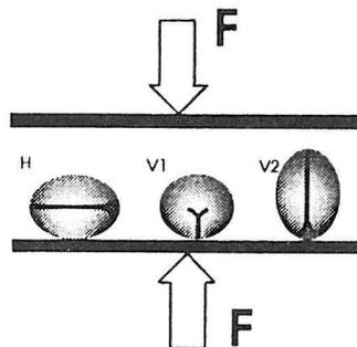
Fig. 1. Three positions of compressed seed distinguished according to internal built of rapeseed: H) dividing plain of cotyledons parallel to compression plates, V1) dividing plain of cotyledons perpendicular to compression plates, V2) dividing plain of cotyledons perpendicular to compression plates with a germ placed on a plate.
