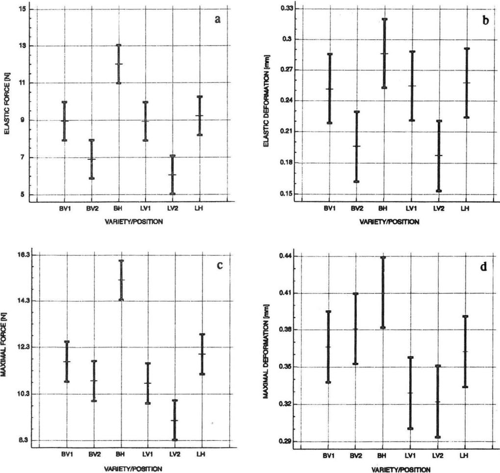
Fig. 3. Mean values with confidence intervals of elastic force (a), elastic deformation (b), maximal force (c), maximal deformation (d) of compressed seeds.
