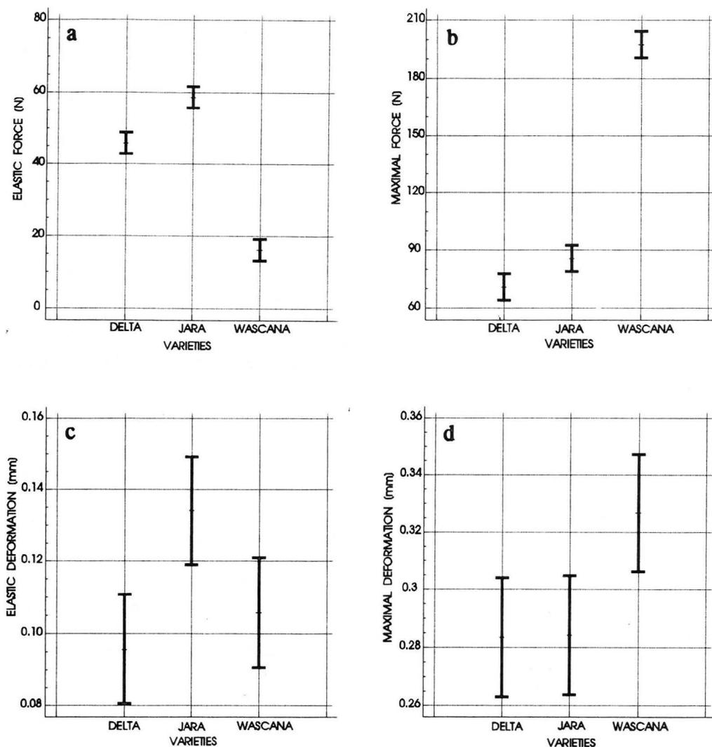
Fig. 3. Mean values with confidence intervals of: elastic force (a), damaging force (b), elastic deformation (c), and damaging deformation (d).
