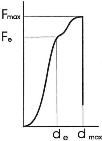
Fig. 1. Characteristic parameters derived from the compression curve.
