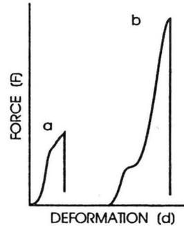
Fig. 2. Typical compression curves of mealy grain (a) and vitreous grain (b).
