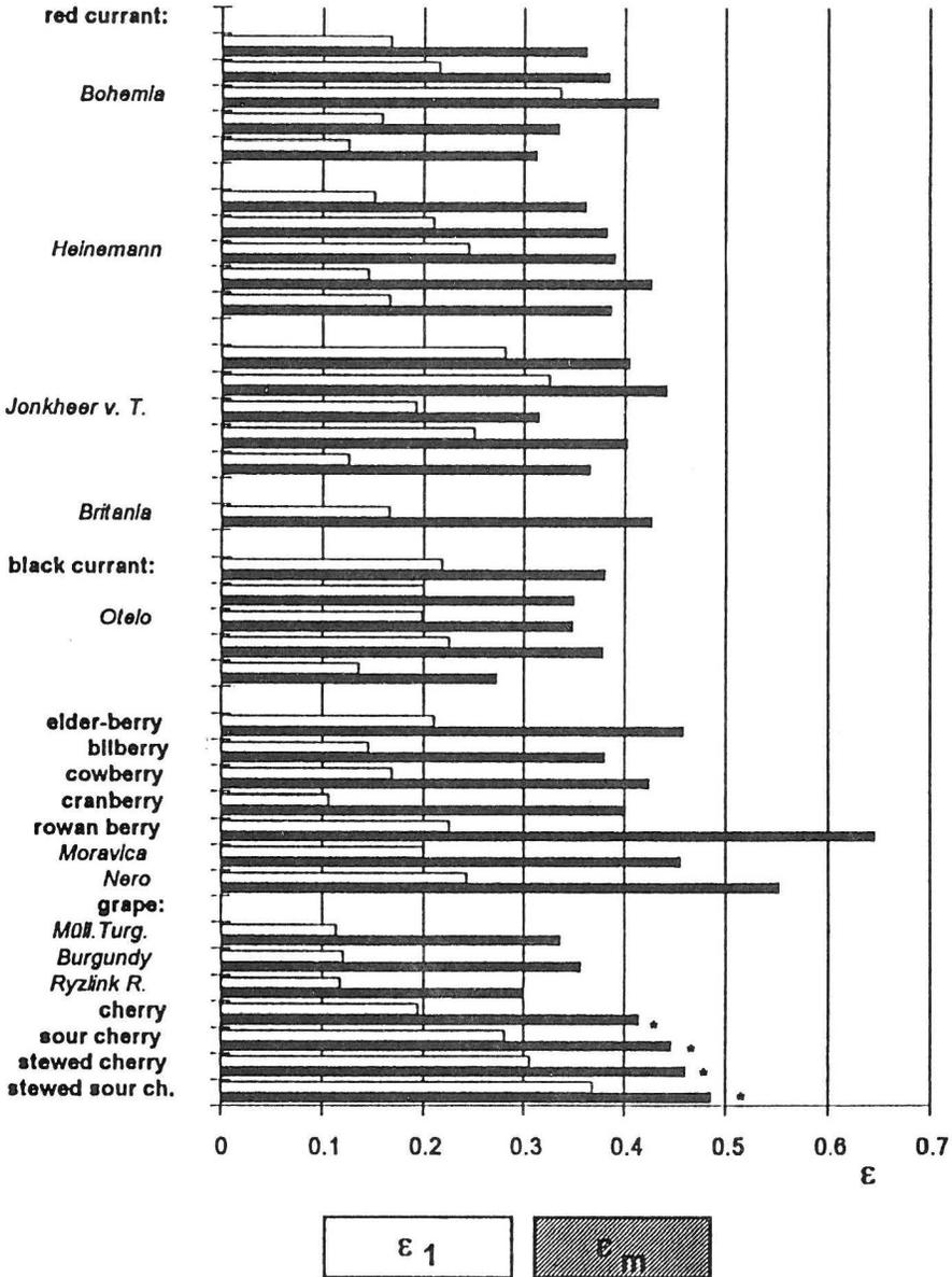
Fig. 4. Mean values of characteristic relative compressions ( $\epsilon_m, \epsilon_1$  in Fig. 1) for different products. The values of  $\epsilon_1$  and  $\epsilon_m$  for different varieties of currant that have been obtained in the whole ripening time (Table 2), [Blahovec, et. al. unpublished data for cherries].
