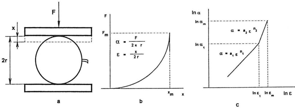
Fig. 1. Compression test of a product between two plates: a - schema of the test; b - dependence of the compression curve on the compression deformation,  $F_m$  and  $x_m$  are coordinates that correspond to the product rupture; c - compression curve plotted in transformed coordinates.
