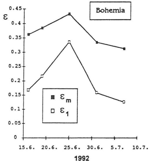
Fig. 3. Examples of changes of toughness ( $\alpha$ ) and/or characteristic relative compressions ( $\epsilon_m, \epsilon_1$  - see Fig. 1) that have been observed in time of ripening.
