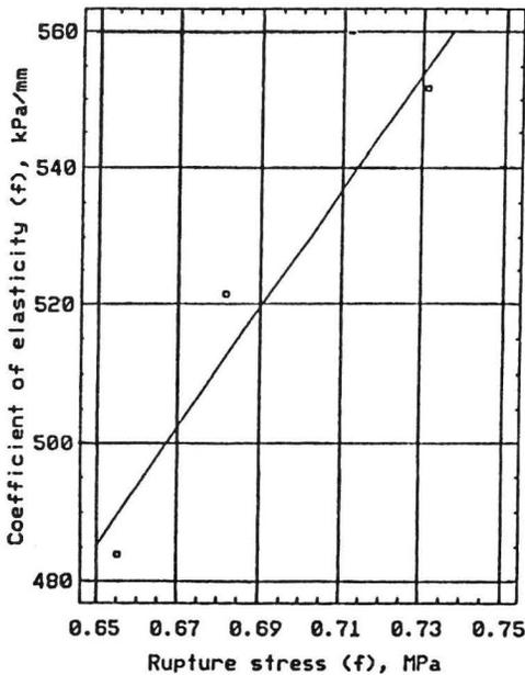
Fig. 5. Coefficient of elasticity (measured by 'f' penetrometer) versus the rupture stress (measured by 'f' penetrometer) for apple:  $y=858.77x - 73.07$ ,  $r=0.9737$ .
