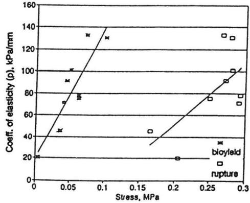
Fig. 3. Coefficient of elasticity (measured by 'p' penetrometer) versus the stress (measured by 'f' penetrometer) for tomato. For bioyield stress:  $y=1216x + 18.94$ ,  $r = 0.876$ ; for rupture stress:  $y=552.5x - 58.55$ ,  $r=0.654$ .
