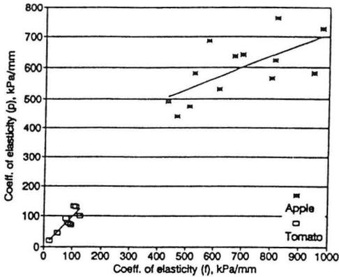
Fig. 1. Coefficient of elasticity (measured by 'p' penetrometer) versus the coefficient of elasticity calculated from the stress-deformation curve (measured by 'f' penetrometer) for tomato and apple. For tomato:  $y=0.963x + 1.377$ ,  $r=0.864$ ; for apple:  $y=0.353x + 354.3$ ,  $r=0.650$ .
