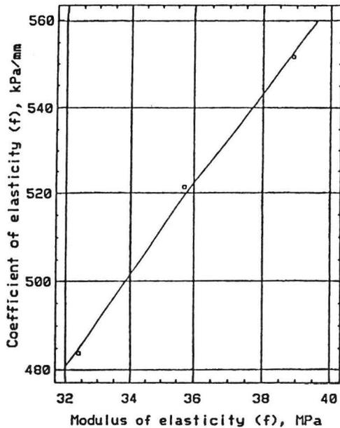
Fig. 4. Coefficient of elasticity (measured by 'f' penetrometer) versus the Young's modulus of elasticity (measured by 'f' penetrometer) for apple:  $y=10.38x + 148.64$ ,  $r = 0.9988$ .
