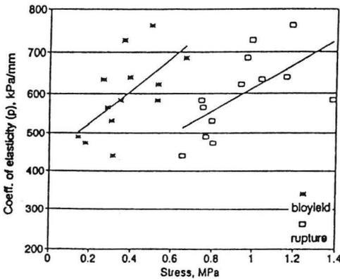
Fig. 2. Coefficient of elasticity (measured by 'p' penetrometer) versus the stress (measured by 'f' penetrometer) for apple. For bioyield stress:  $y=406.3x + 444.5$ ,  $r=0.626$ ; for rupture stress:  $y=285.6x + 327.8$ ,  $r=0.627$ .
