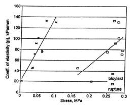
Fig. 3. Coefficient of elasticity (measured by 'p' penetrometer) versus the stress (measured by 'f' penetrometer) for tomato. For bioyield stress: y=1216 x +18.94, r = 0.876; for rupture stress: y=552.5 x - 58.55, r=0.654.
