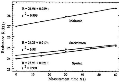
Fig. 3. Apple electrical resistance versus measurement time in commercial harvest date.
