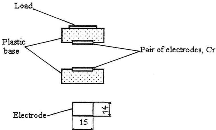
Fig. 2. Experimental probe sensor for sample measurements.
