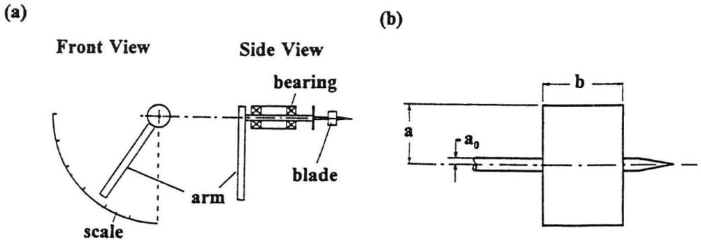
Fig. 1. Principle of operation of Massey Twist Tester. a - general layout, b - enlargement of blade.
