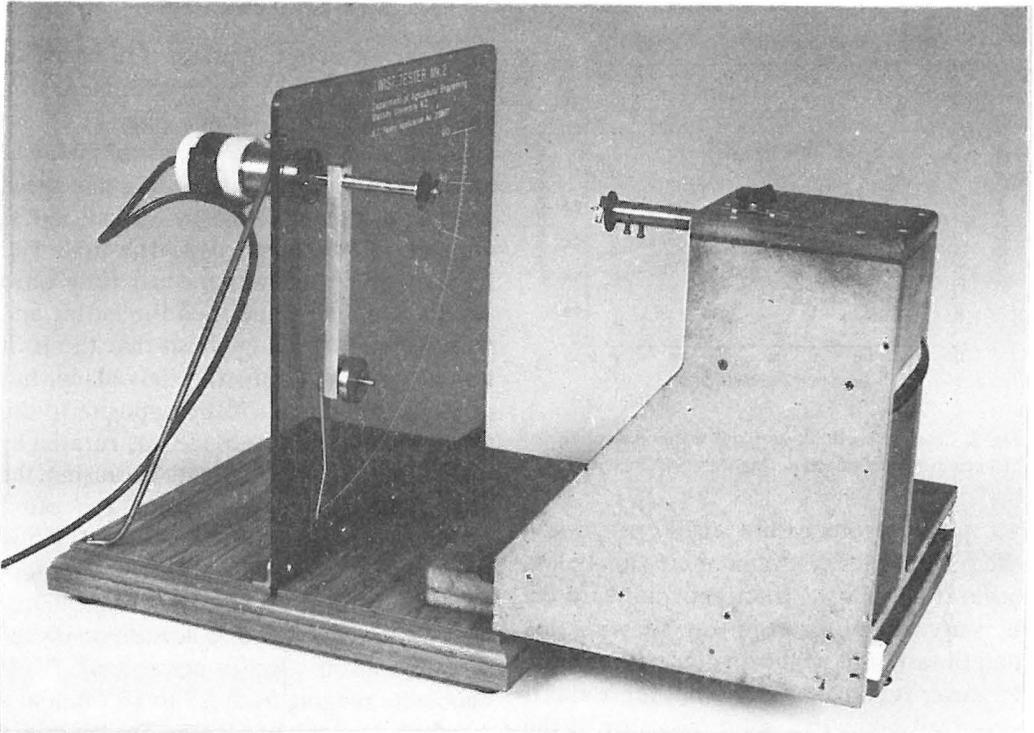
Fig. 4. Motor driven Twist Tester.
