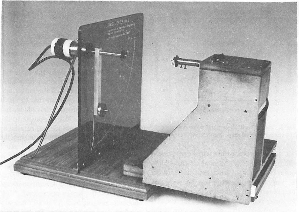
Fig. 4. Motor driven Twist Tester.
