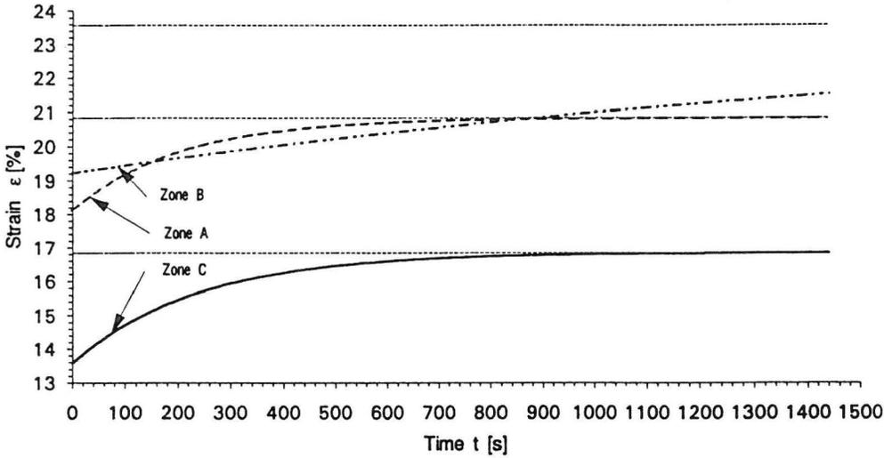
Fig. 2. Theoretical curves of creep for A, B, C zones of sugar beet root.
