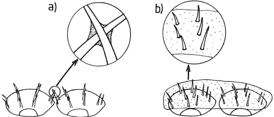
Fig. 1. Contact glue joint (a) and coat glue joint (b).
