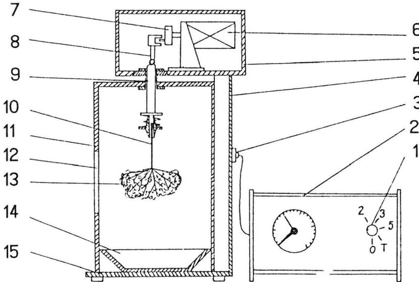
Fig. 2. Shattering set: 1 - potentiometer, 2 - power with frequency control, 3 - connection, 4 - pillar, 5 - drive casing; 6 - direct current motor, 7 - circular cam, 8 - connective rod, 9 - slider, 10 - shoot in holder, 11 - shattering chamber, 12 - sight-glass, 13 - seedhead, 14 - container, 15 - base plate.
