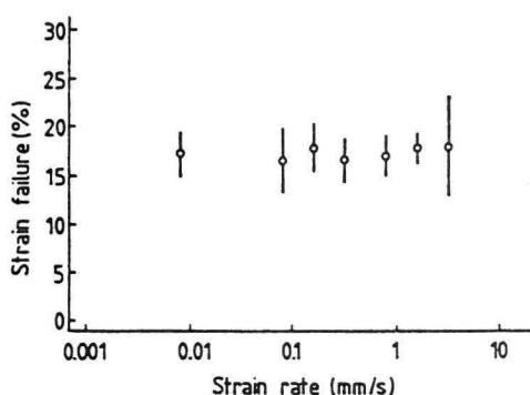
Fig. 2. Influence of strain rate on relative strain failure.
