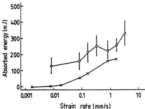
Fig. 1. Influence of strain rate on absorbed energy (o) and calculated energy (x).
