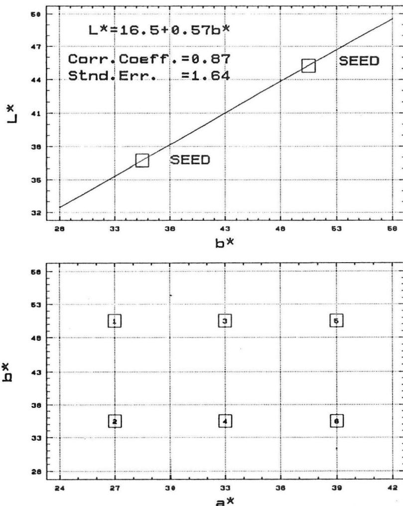
Fig. 2. Colour coordinates of seeds of colour classes projected on to  $b^*$ ,  $L^*$  and  $a^*$ ,  $b^*$  colour plane.
