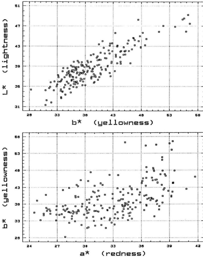
Fig. 1. Colour coordinates of 210 samples of ground paprika projected on to  $b^*$ ,  $L^*$  and  $a^*$ ,  $b^*$  colour plane.
