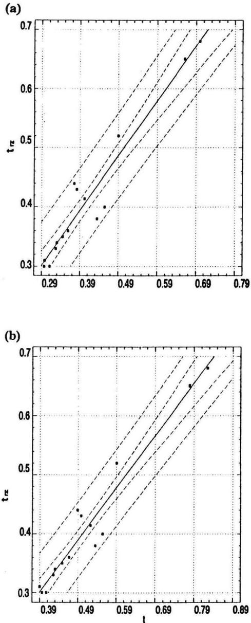
Fig. 1. Regression of experimental freezing time ( $t_{fz}$ ) of potato in relation to time ( $t$ ) calculated under Cleland's model; properties acc. to [14] (a) and [1] (b).
