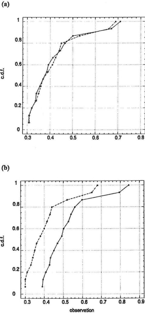
Fig. 2. Cdf plot of experimental freezing time ( $t_{TZ}$ ) of potato and time ( $t$ ) predicted after Cleland's model; properties acc. to [14] (a) and [1] (b).  $t_{TZ}$  - solid line,  $t$  - dashed line.
