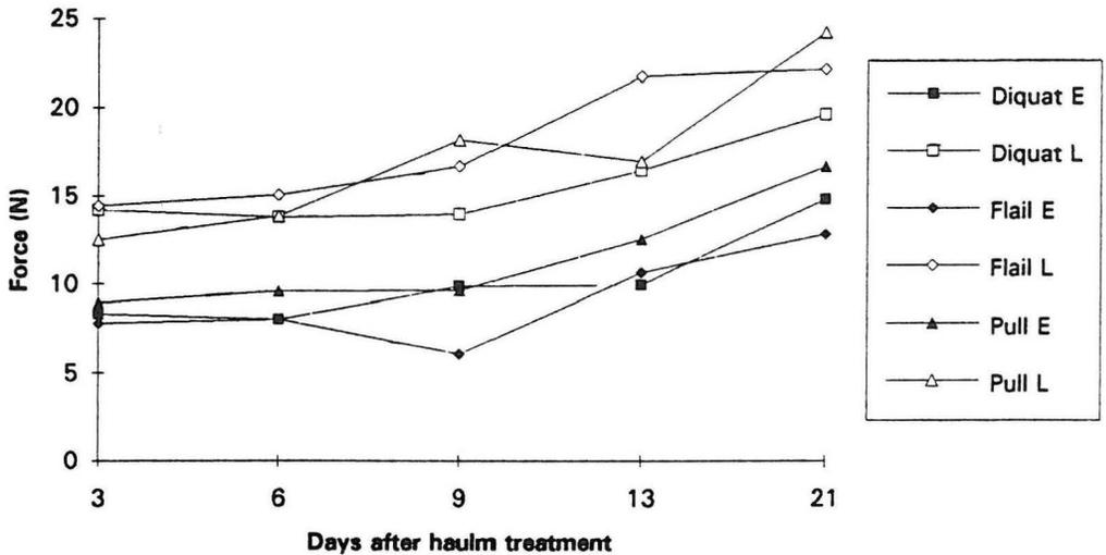
Fig. 5. The effect of the method of haulm treatments on skin strength.
