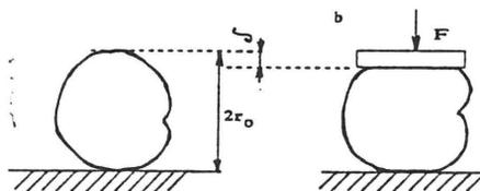
**Fig.1.** Compression of a round product between two plates, a - initial form of the product with characteristic dimension  $2r_0$ , b - the product compressed by the force  $F$  between two plates,  $\delta$  - compression of products.
