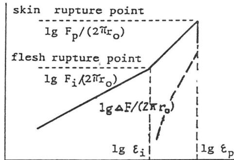
Fig. 3. Schematical drawing of a typical compression curve of a berry-like fruit compressed between two plates (full line). Function  $\log [(F-\Delta F)/(2\pi r_o)]$  is denoted by the dashed line.
