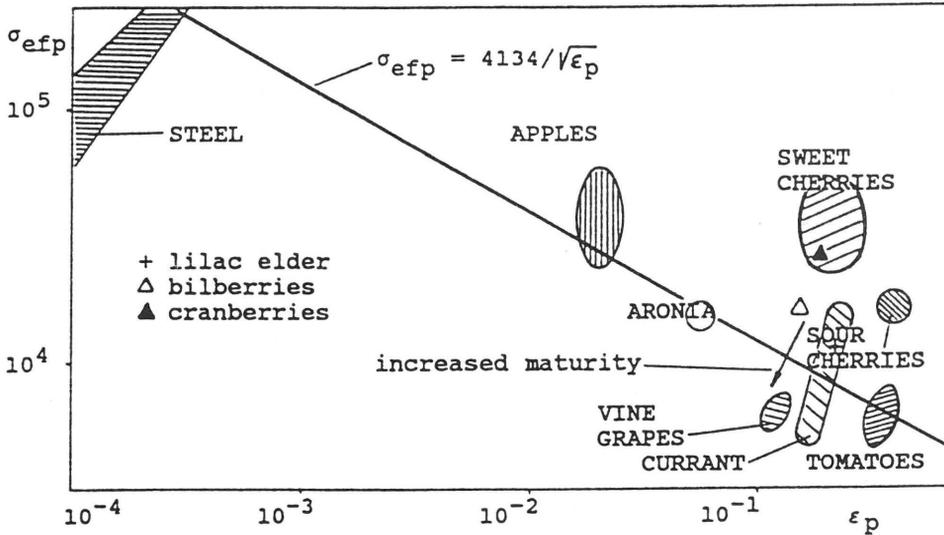
Fig. 2. Critical values of effective stress ( $\sigma_{efp}$ ) in relation to critical values of relative compression ( $\epsilon_p$ ) for different agricultural round products and steel spheres. Critical point is identified with the beginning of anelastic behaviour of the compressed product and/or sphere in this case.
