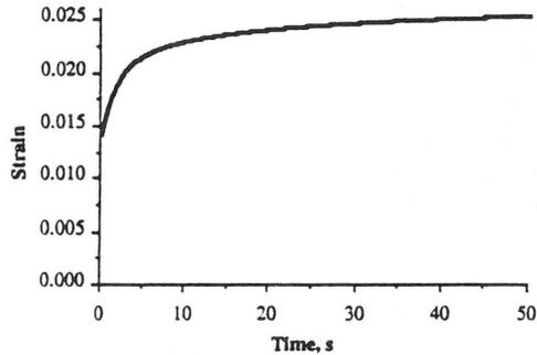
**Fig. 3.** Numerically determined creep response of a generalized Maxwell model using the viscoelastic parameters in Table 1. The model was subjected to a constant stress load of  $\sigma_0$ .
