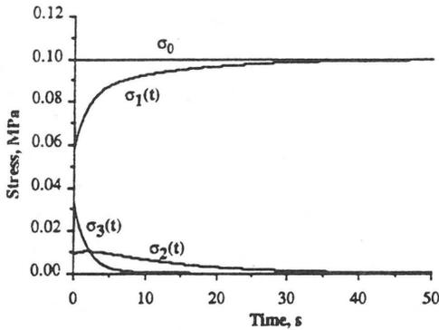
Fig. 4. Numerically determined stress response of each element of a generalized Maxwell model using the viscoelastic parameters in Table 1. The model was subjected to a constant stress load of  $\sigma_0$ .
