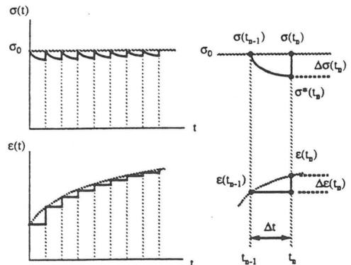
Fig. 2. Incremental changes of stress and strain in each discrete time interval.
