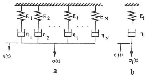
Fig. 1. Generalized Maxwell model (a) and the *i*th simple Maxwell element (b).
