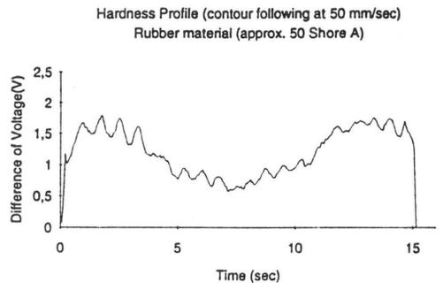
Fig. 7. Continuous hardness measurement at 50 mm/s.
