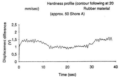
Fig. 6. Continuous hardness measurement at 20 mm/s.
