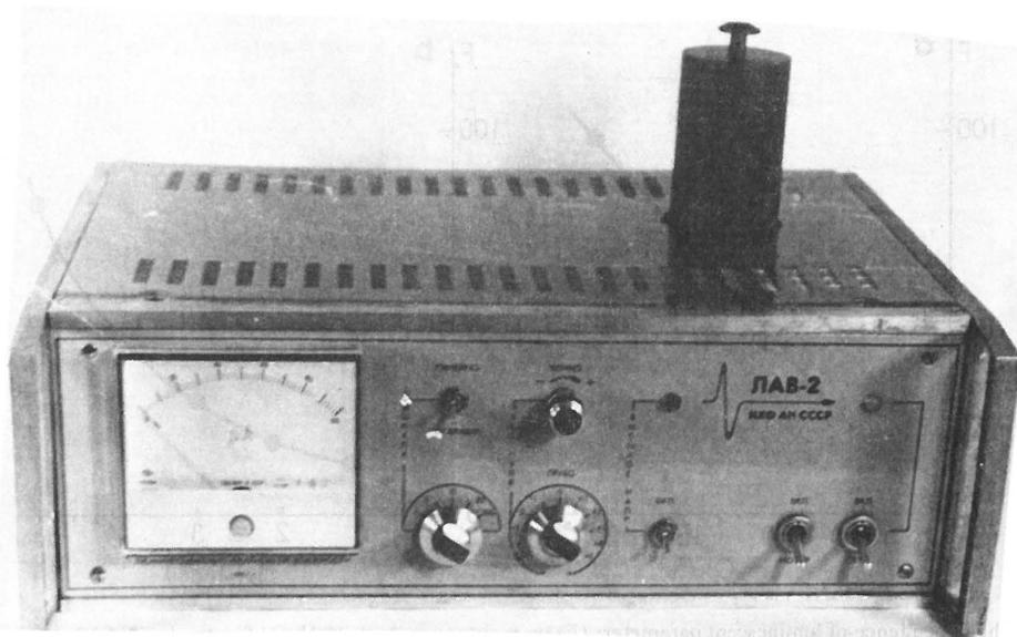
Fig. 3. Home-made luminescent analyser of moisture.
