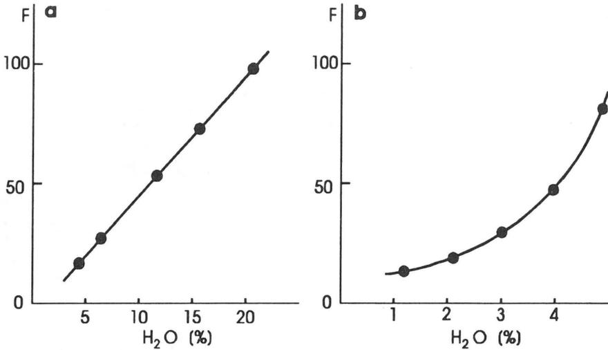
Fig. 5. The dependence of luminescent parameters (F) on moisture content (% H<sub>2</sub>O) for dried milk (a), and grain (b). T = 23 °C.
