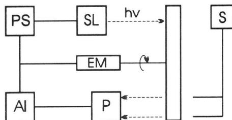
Fig. 2. Block-scheme of luminescent analyser. PS-power supply, SL-source of light, EM-electromechanical modulator, P- photomultiplier, AI - analog indicator, S-sample.
