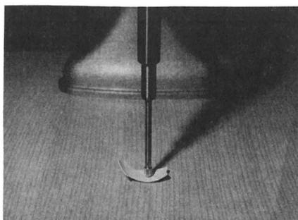
Photo 3. Shell thickness measurement.
