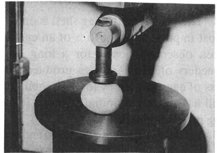
Photo 2. Measurement of the power needed for burst of egg shell.
