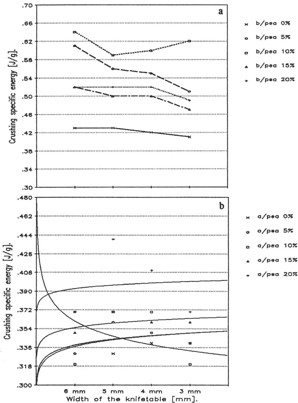
Fig. 4. The influence of the width of the knife table on the specific crushing energy. Die 3.5 mm, mixture B/b (a); Die 3.5 mm, mixture C/a (b).
