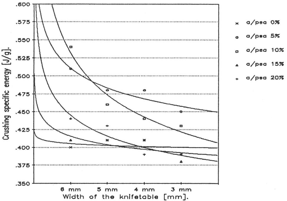
Fig. 7. The influence of the width of the knife table on the specific crushing energy. Die 4 mm, mixture C/a.
