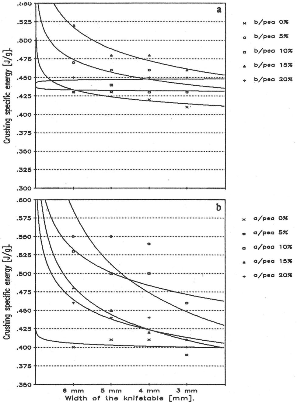
Fig. 5. The influence of the width of the knife table on the specific crushing energy. Die 3.5 mm, mixture C/b (a); Die 4 mm, mixture A/a (b).
