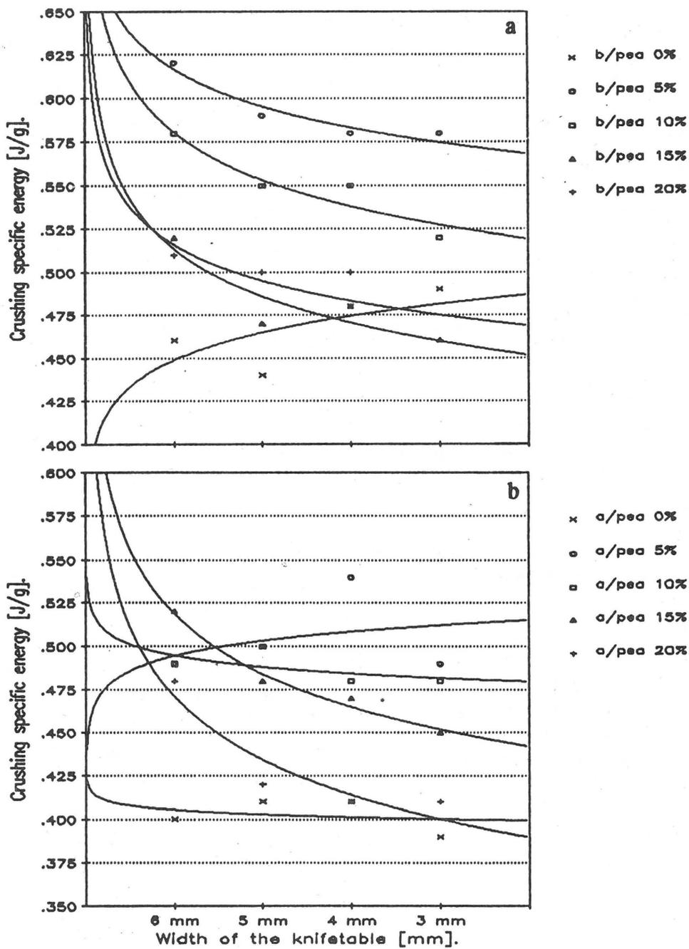
Fig. 6. The influence of the width of the knife table on the specific crushing energy. Die 4 mm, mixture A/a (a); Die 4 mm, mixture B/b (b).
