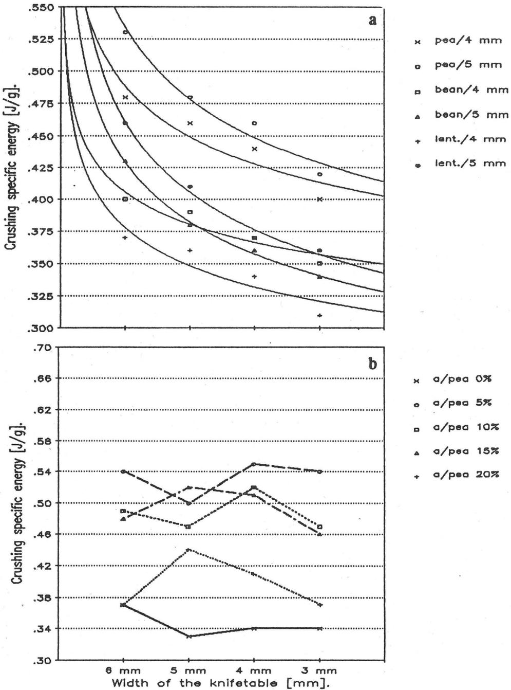
Fig. 2. The influence of the width of the knife table on the specific crushing energy. Pulses rate 20 % (a); Die 3.5 mm, mixture A/a (b).
