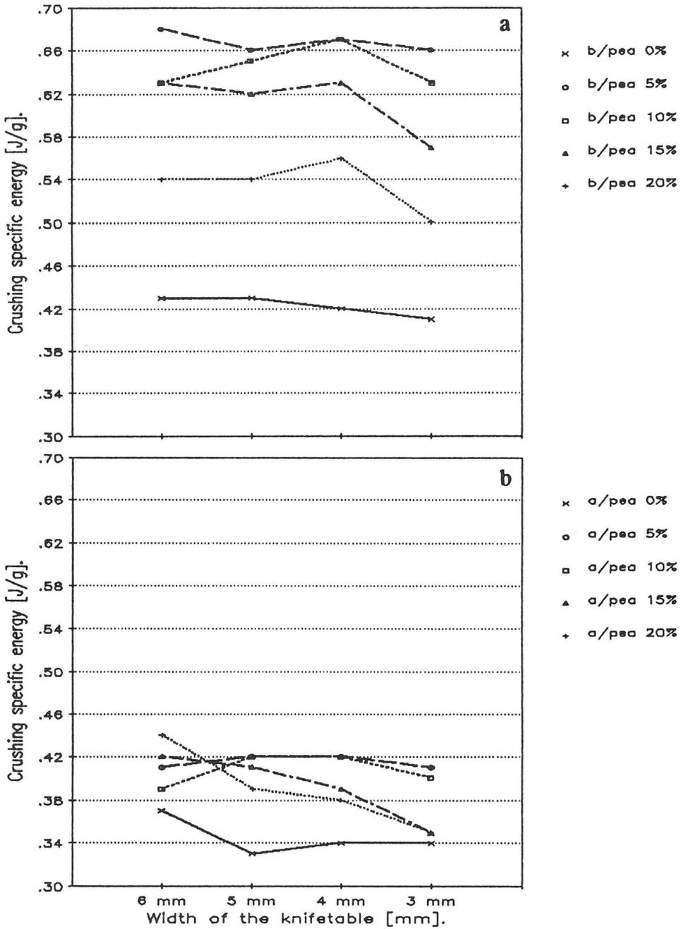
Fig. 3. The influence of the width of the knife table on the specific crushing energy. Die 3.5 mm, mixture A/b (a); Die 3.5 mm, mixture B/a (b).
