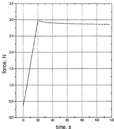
Fig. 2. Stress relaxation in flax fibres (variety Marina, experiment No. 0003) Test data: initial load 3 N, deformation speed 0.4 mm/min, time basis 100 s, load range 50 N.
