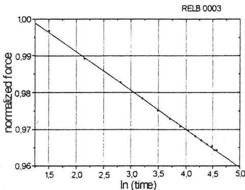
Fig. 3. Normalized stress relaxation curve of flax fibre with regression line (variety Marina, experiment No. 0003). Linear regression data:  $Y=A+B \cdot X$ ,  $A=1.01211$ ,  $B=-0.01052$ ,  $R=-0.99959$ .
