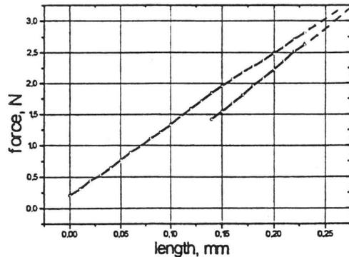
Fig. 1. Force-elongation-diagram of flax fibre (variety Marina, exp. No. 0007). Test data: maximal force 3 N, deformation speed 0.4 mm/min, load range 50 N.
