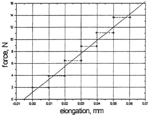
Fig. 4. Force-elongation-diagram of the Zwick testing machine (Institut für Landtechnik, Bonn). Test data: maximal force 14 N, load range 50 N, deformation speed 0.04 mm/min, minimal length resolution 0.01 mm.
