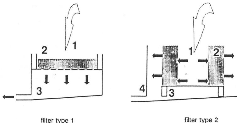
Fig. 1. Working positions of the filters. 1 - sewage influx; 2 - wheat straw mattress; - efflux; 4 - box.
