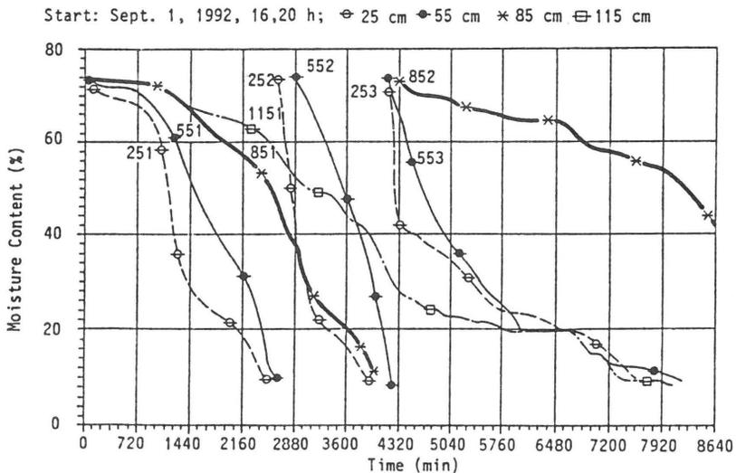
Fig. 4. Drying curves of hops layers of different thickness in the period 1-8 September 1992.
