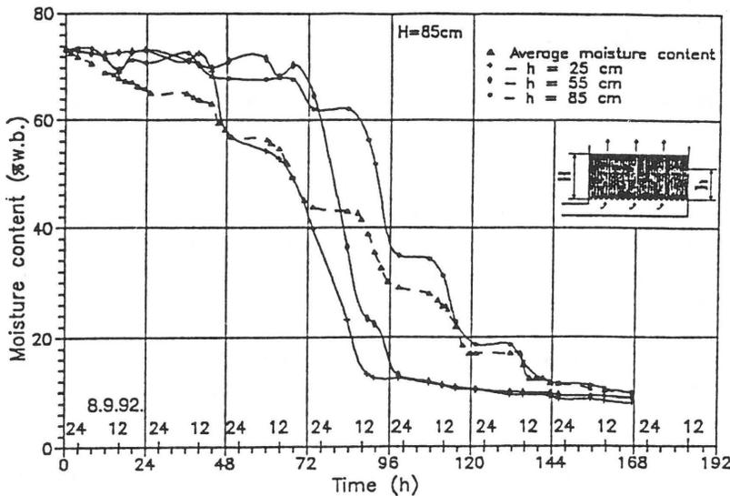
Fig. 5. Drying of hops in different segments within the 85 cm layer.
