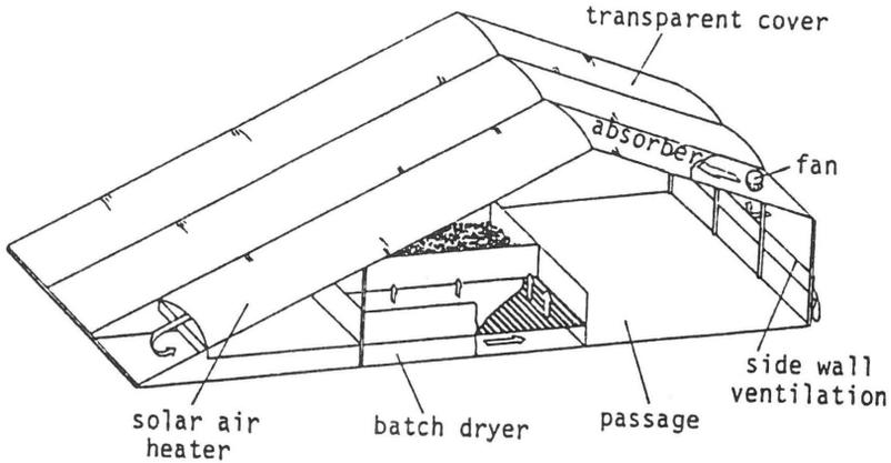
Fig. 1. Experimental solar dryer-plastic house.
