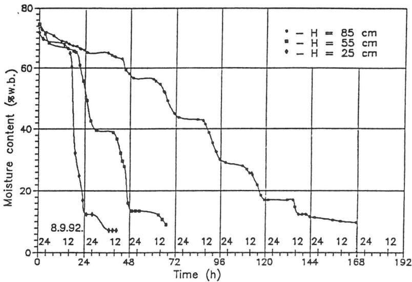
Fig. 3. Drying of hops layers of different thickness.
