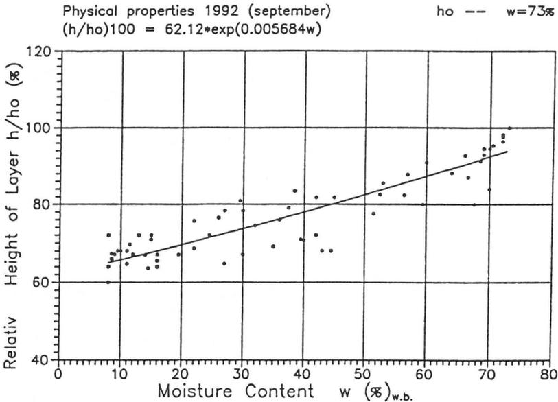
Fig. 6. The relative reduction of the hops layer's initial height during drying.
