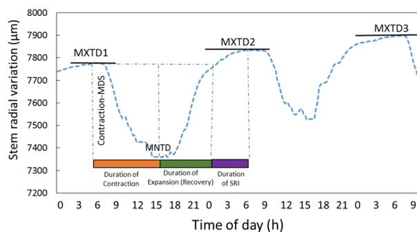
**Fig. 1.** Schematic of the diel course of trunk diameter, the maximum daily shrinkage (MDS), the stem radial increment (SRI), and the durations of the contraction, recovery and SRI phases are shown. The maximum (MXTD) and the minimum trunk diameter (MNTD) are indicated.
