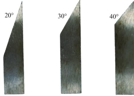
**Fig. 3.** Different blade angles.
