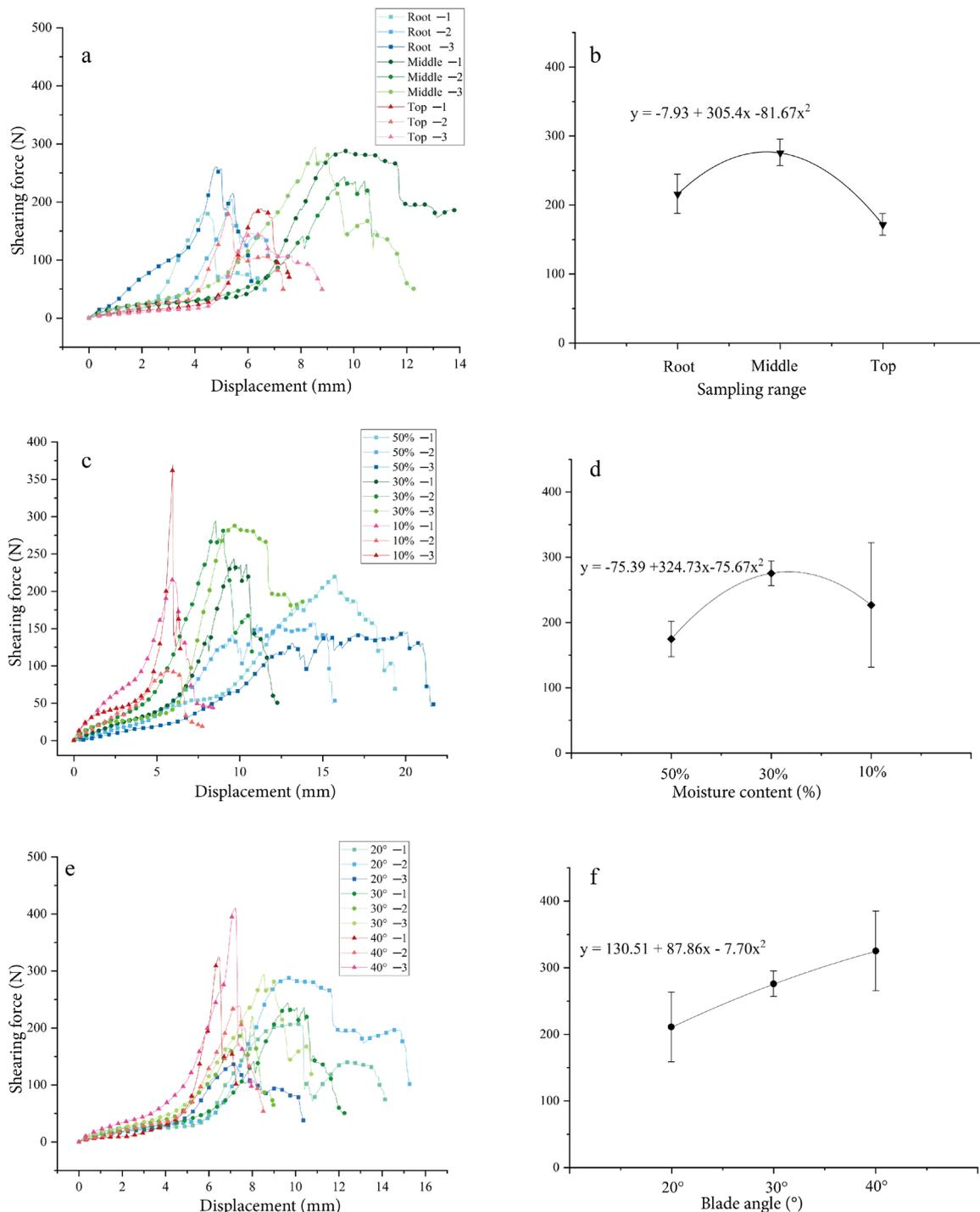
**Fig. 5.** The influence of various factors on shearing characteristics: (a) curves of shearing force and displacement under sampling range, (b) effect of the sampling range on the shearing force, (c) curves of shearing force and displacement under moisture content, (d) effect of the moisture content on the shearing force, (e) curves of shearing force and displacement under blade angle, (f) effect of the blade angle on the shearing force.
