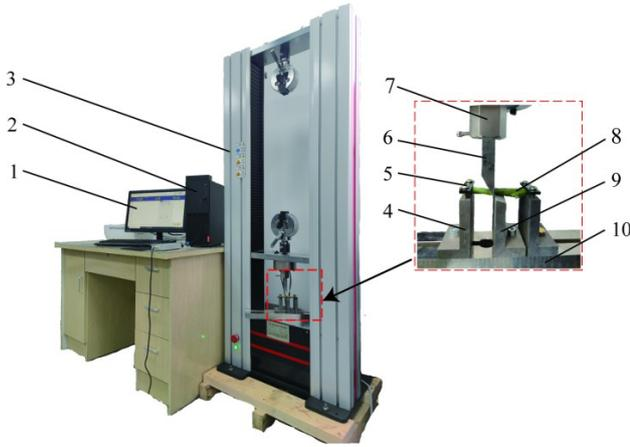
**Fig. 2.** Tomato stem shear test bench: 1 – display, 2 – computer, 3 – WDW-20 microcomputer-controlled electronic universal testing machine, 4 – block, 5 – press plate, 6 – moving knife, 7 – tool chuck, 8 – stem sample, 9 – fixed knife, 10 – pad block adjustment track.
