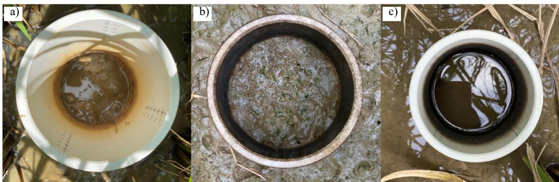
**Fig. 5.** Inside view of soil chamber collars: a) immediately after drainage (14 September), b) under drainage conditions, and c) re-submerged after rainfall (23 September).
