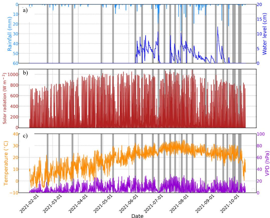
**Fig. 3.** Seasonal variations of meteorological variables at the study site from February to October 2021: a) 30 min sum of rainfall and average of water level, b) solar radiation, and c) air temperature and VPD. The grey vertical lines indicate the days when soil CO<sub>2</sub> efflux observations were conducted using the chamber method.
