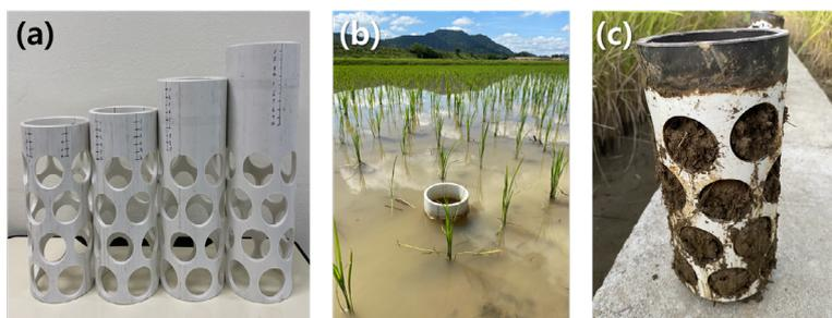
**Fig. 2.** Soil collars inserted into the paddy soil: a) 4 different heights of collars, b) soil collars inserted around rice, and c) roots inside the collar removed just before harvest.
