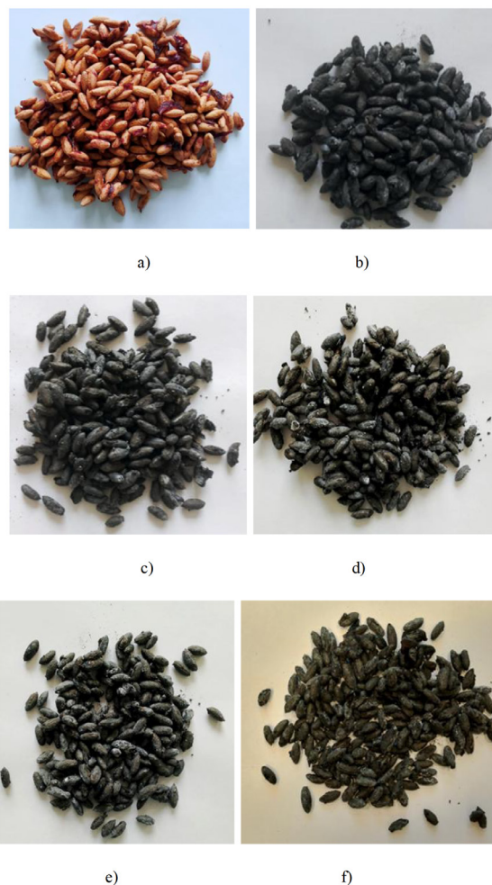
Fig. 3. Cornelian cherry seeds and prepared biochar: a) no thermal treatment; pyrolysis (min): b) 2, c) 4, d) 6, e) 8, f) 10.
