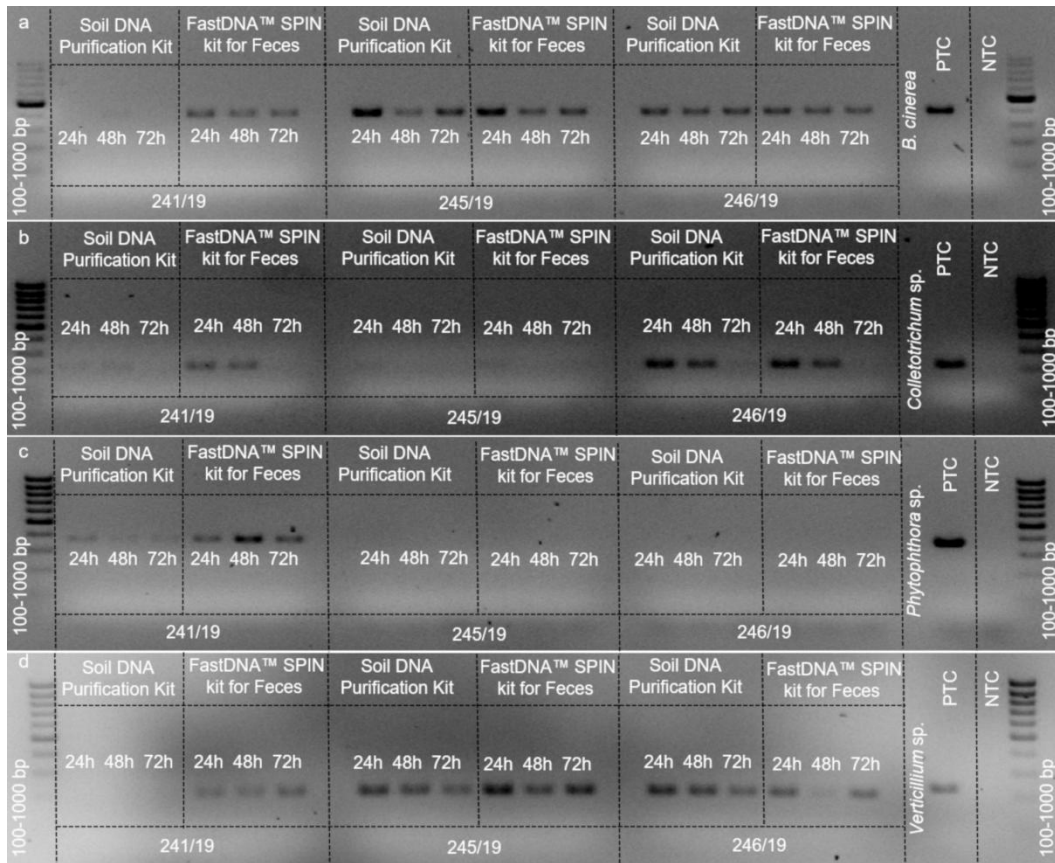
Figure S21. The specificity of the primer on naturally infected strawberry fruit. PCR amplification using B. cinerea (a), Colletotrichum sp. (b), Phytophthora sp. (c), and Verticillium sp. (d) specific primers in strawberry fruit (241/19; 245/19; 246/19) naturally infected incubated at 24°C for 24, 48, and 72 hours using 2 different kits of DNA extraction. Gel agarose 2% with 100-1,000 bp ladder. NTC means non-template control, and PTC is positive-template control ( B. cinerea – G277/18; Colletotrichum sp. – G171/18; Phytophthora sp. – G408/18; Verticillium sp. – G296/18). The sample 245/19 came from a healthy plant; whereas 241/19 and 246/19 were collected from symptomatic plants diseased by pathogens. The replications are presented in the Figure S22.
