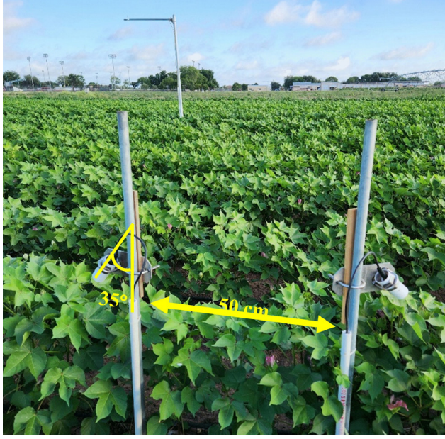
Fig. 2. Details of the installation of the infrared radiometer sensors in the cotton field at the Uvalde Research Center in 2025. Shown in the background is the NR-Lite2 net radiometer mounted on a metal pole.
