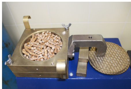
Fig. 1. Circular shear cell 10 cm in diameter used in this research for the direct shear tests carried out with samples of wood pellets.
